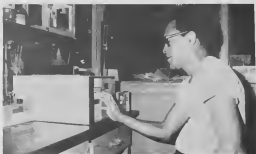
Lab Assistant F. Holmond is running a test through push-button action for sulfur content on the new X-Ray Sulfur Analyzer.
